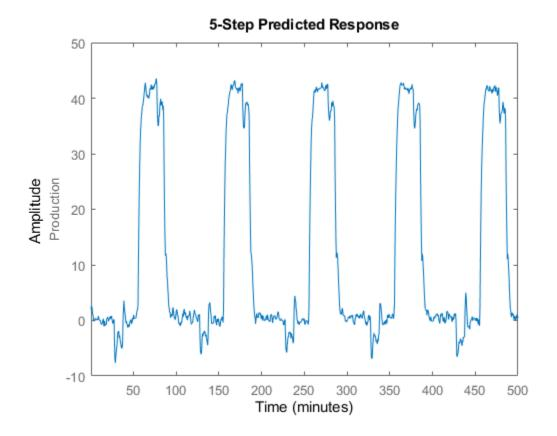
Compare the predicted output values with the measured output values. The third argument of compare specifies a five-step-ahead prediction. When you do not specify a third argument, compare assumes an infinite prediction horizon and simulates the model output instead.
