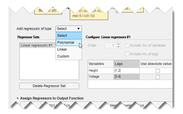
This action adds a polynomial regressor set called **Polynomial regressors #1** to the list of regressor sets. By default, this set is configured to generate regressors of order 2, as shown in the configuration panel.
