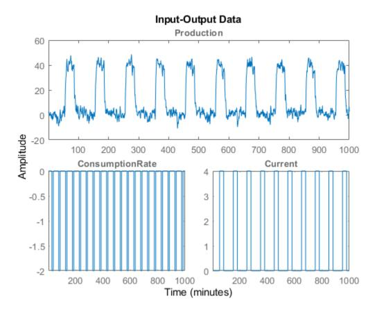
The bottom axes show inputs ConsumptionRate and Current, and the top axes show the output ProductionRate.
