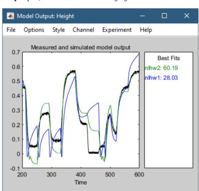
This action adds the model nlhw2 to the **System Identification** app and updates the **Model Output** plot, as shown in the following figure.
