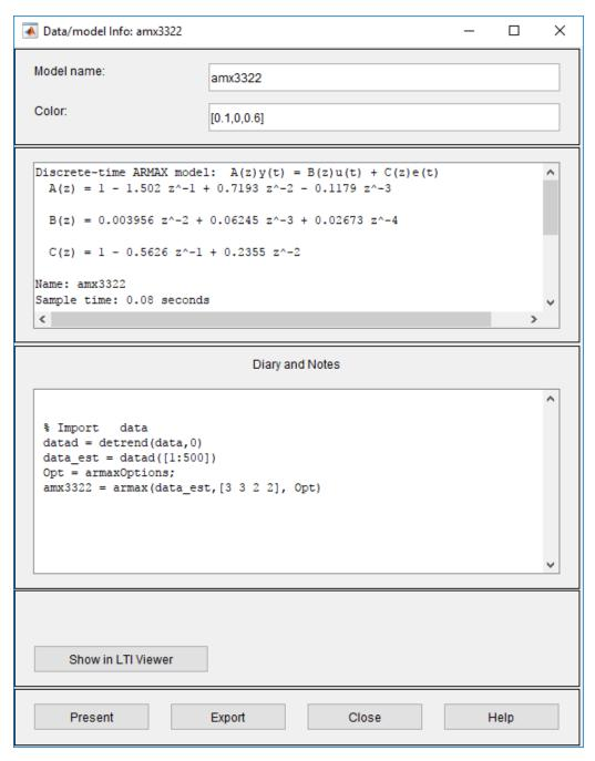
The noneditable area of the Data/model Info dialog box lists the parameter values correspond to the following difference equation for your system:
