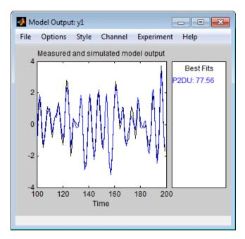
The System Identification Toolbox software uses input validation data as input to the model, and plots the simulated output on top of the output validation data. The preceding plot shows that the model output agrees well with the validation-data output.
