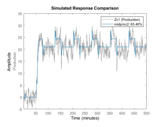
The plot shows that the model output maintains reasonable agreement with the validation-data output.
