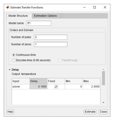
4 Click **Estimate** to add a transfer function model called tf1 to the System Identification app. You can view the output of the estimation of the transfer function model in comparison with the estimations of other models, in the Model output window.
