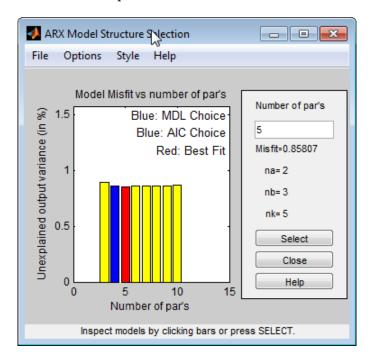
**Note** The Rissanen MDL and Akaike AIC criteria produces equivalent results and are both indicated by a blue rectangle on the plot.
