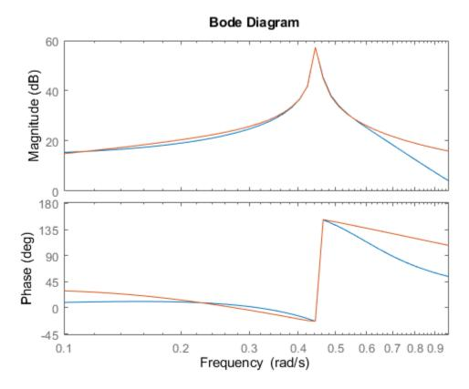
The FRD model is generated from the fifth-order system sys0. While sys, a third-order approximation, does not capture the entire response of sys0, it captures the response well until approximately 0.6 rad/s.
