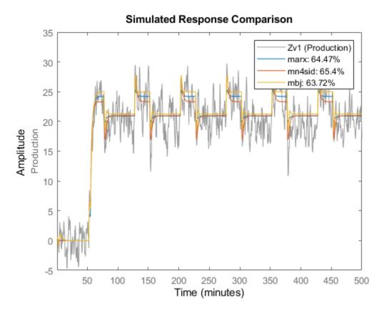
compare plots the measured output in the validation data set against the simulated output from the models. The input data from the validation data set serves as input to the models.
