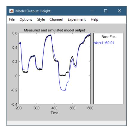
The **Best Fits** area of the model output plot shows the agreement between the model output and the validation-data output using a normalized root mean squared (NRMSE) metric of goodness of fit. The agreement is poor in the 400-500 time span.
