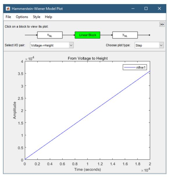
4 In the **Choose plot type** list, select Bode. This action displays a Bode plot of the linear transfer function.
