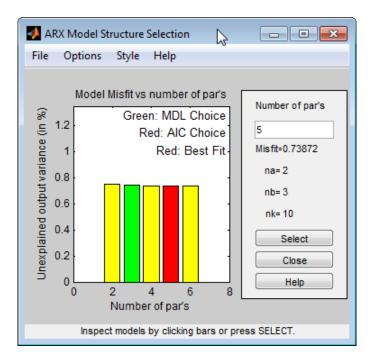
**Note** The Akaike AIC and the overall best fit criteria produces equivalent results. Both are indicated by the same red rectangle on the plot.
