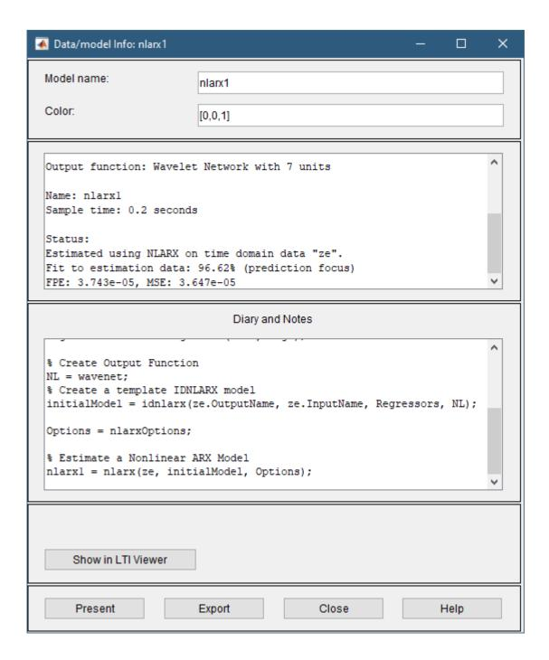
**Note Fit (%)** is computed using the estimation data set with prediction focus. and not the validation data set. However, the model output plot in the next step compares the fit to the validation data set. To see how well the model can simulate the response of an independent validation dataset, use the **Model Output** plot, as discussed in the following step.
