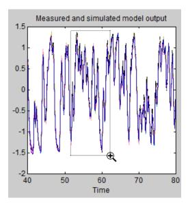
Releasing the mouse magnifies this region and shows that the output of all models matches the validation data well.
