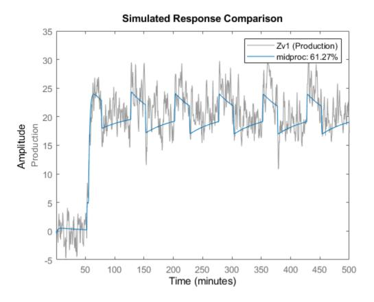
The plot shows that the model output reasonably agrees with the measured output: there is an agreement of 60% between the model and the validation data.
