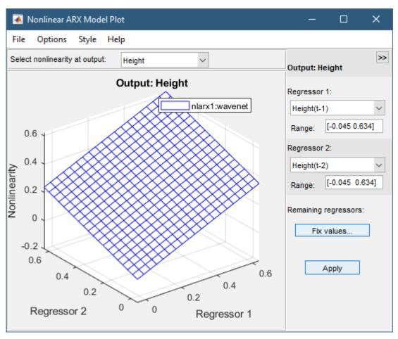
In the Nonlinear ARX Model Plot window, set **Regressor 1** to Voltage(t-1). Set **Regressor 2** to Voltage(t-2). Click **Apply**.
