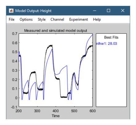
The model nlhwl does not validate well. The fit to zv.OutputData is poor.
