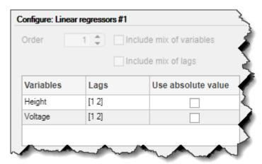
The regressor assignment table **Assign Regressors to Output Function** lists the regressor names and the regressor assignments to the output function components.
