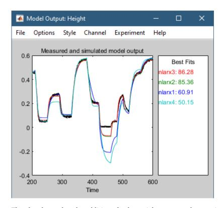
The plot shows that the addition of polynomial regressors has not improved the generalization ability of the model. That is, the model does not provide a better fit between the model output and the measured output for independent validation data. This result is typically the scenario with overfits, that is, when the model contains more regressors than absolutely required.
